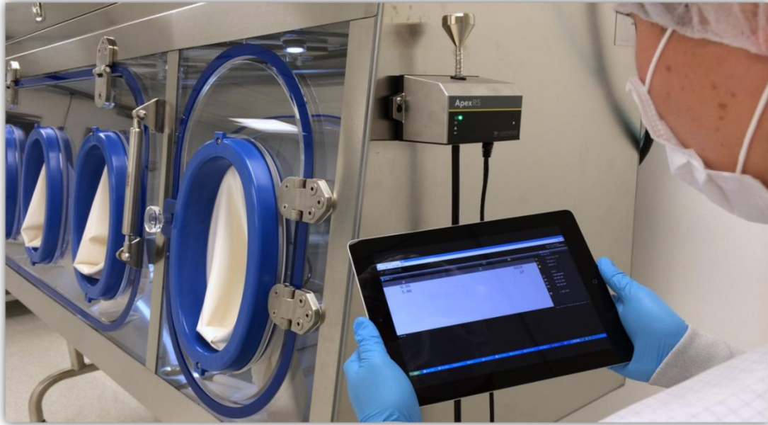
End User validation (PQ) of remote Particle Counter location in a Cleanroom – Grade B Environment.
